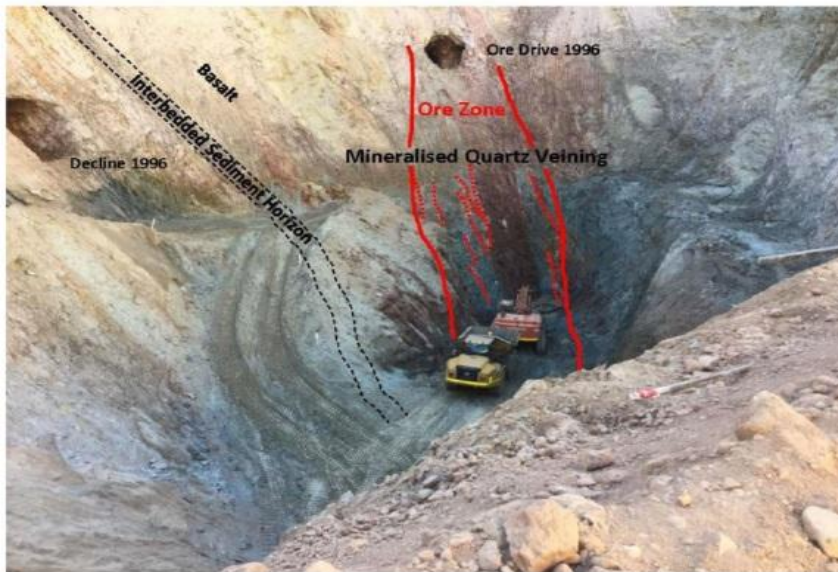
Figure 9: Location of new adit on north wall of Eureka pit showing ore zone, excavator and truck at pit floor in 2018 during Tribute Mining.
